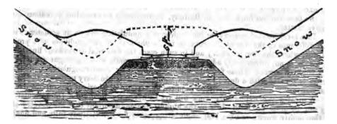
The snow is supposed to be five feet in perpendicular depth, the dotted line show where its surface would be, supposing the Railway to have been closed all winter, and the full line shows where the snow would be deposited along the side, on being cast to the right and left from the rail track.
